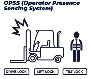
The OPSS System restricts driving, lifting and tilting, and it kicks in automatically when the operator leaves the seat to prevent accidents. It operates in conjunction with the auto parking brake to contribute to a safer workplace.
