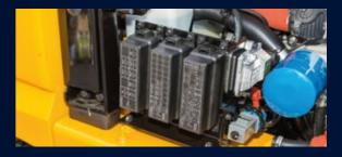
All fuses and relays are centralized in three boxes with **enhanced waterproof and dustproof protection IP65**. The boxes themselves are located behind the side cover panel for **quick access**. **Parts & Warranties**
