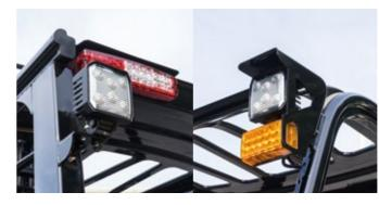
The LED lights offer the optimal visibility under any conditions.
