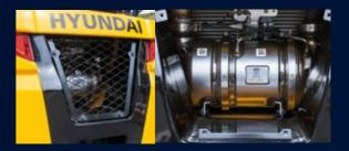
For greater convenience, the counterweight opening has been made as large as possible. This **eliminates the need to remove the counterweight** for inspection or exchange of the after-treatment device.
