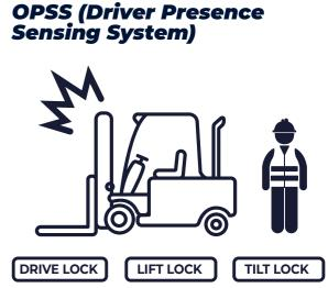
The OPSS System restricts driving, lifting and tilting, and it kicks in **automatically when the driver leaves the seat** to prevent accidents. It operates in conjunction with the auto parking brake to contribute to a safer workplace.
