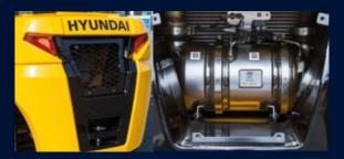
For greater convenience, the counterweight opening has been made as large as possible. This **eliminates the need to remove the counterweight** for inspection or exchange of the aftertreatment device.
