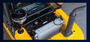
The radiator can be accessed by a removable top cover to **reduce the downtime when checking and refilling the coolant or cleaning the radiator.**
