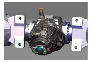
The parking brake operates automatically when the power is disengaged in order to prevent accidents caused by human error. Hill Start Assist Control (HAC) prevents backsliding when restarting on a slope.
