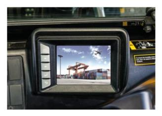
The rear view camera is integrated in the cluster and can be **activated using a button or automatically while driving backwards.**
