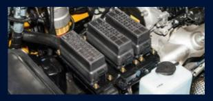
All fuses and relays are centralised in three boxes with **enhanced waterproof and dustproof protection IP65**. The boxes themselves are located under the engine hood for **quick access**.
