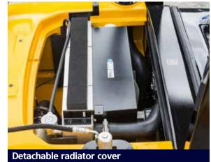
The plastic tool-less radiator sub-hood on top of the counterweight separated from the main hood reduces the downtime for checking the cooling water level and makeup.
