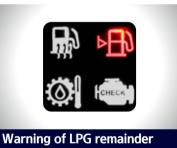
When the pressure inside the LPG tank drops below the setting due to consumption of fuel during drive, the Fuel Symbol lamp lights on the cluster to prevent any inconvenience caused by the exhaustion of LPG during work.
