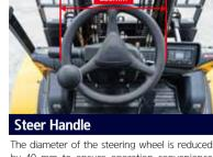
The diameter of the steering wheel is reduced by 40 mm to ensure operation convenience and reduce the driver's fatigue. Furthermore, applying new functional devices and optimal turning function prevents jamming, heavy feeling, and noise resulting from sudden handling.
