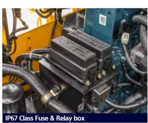
The fuse and relay, which are vulnerable to contamination, are installed in water- and dust-tight box that is in turn installed in the engine compartment to reduce the downtime for maintenance.
