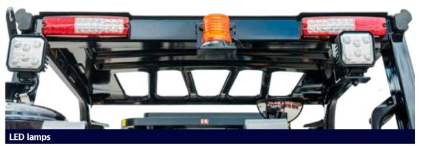
LED lamps include headlamp, rear work lamp, and combination lamp, which provide higher luminance than halogen lamps. LED lamps with semi-permanent service life apply to ensure good view and visibility during night work.
