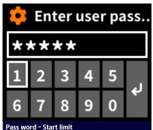
A function of password input on the cluster applies for preventing safety accident or damage that may take place on the equipment when any unauthorized operator or administrator operates the equipment. (Up to ten passwords are allowed.)
