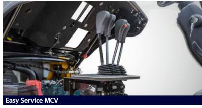
MCV, one of the major functional parts of the hydraulic system, is installed in a horizontal direction to allow the adjustment of hydraulic pressure and exchange of spool without opening the MCV assembly.
