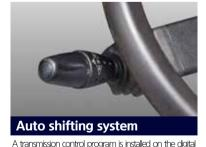
A train should program is installed on the object of the object of the object of the first and second duster for automatic gear shifting of the first and second gears depending on the rotation rate of transmission out shaft to prevent the reduction of service life of transmission caused by forced start at forward second gear. (Switching to manual mode allowed)
