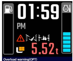
Cargo weight measurement function configured with pressure sensor of lift line and cluster program provides real-time indication of weight of lifted cargo and prompts a warning on the cluster in case of overloading to remind the operator of safety.
