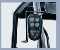
The new efficiency lighting system employs LED illuminant and new type reflector to reduce energy consumption, improve significantly illumination performance and evaluate work time.
