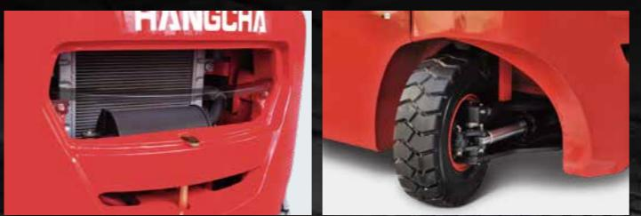
► Extra capacity combined radiator with serpentine wave and optimized heat dissipation channel enhance the heat dissipation capability to keep engine reliability even in heavy-duty applications.
