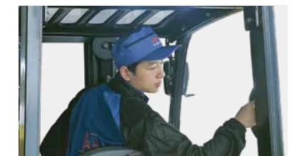
► An optional rear-pillar assist grip with a horn button enhances safety of operator while traveling in reverse.
