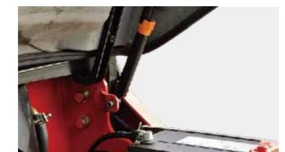
► The locking device of the engine hood damper and parking brake help add to safety.
