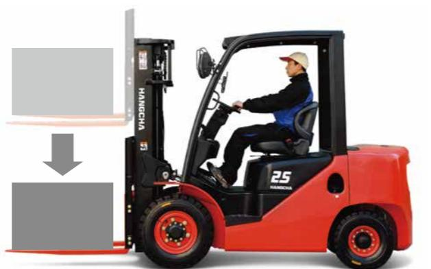
► The operator presence sensing system incorporates lifting/tilting and traveling locking function. When the operator leaves the seat, the system automatically locks lifting / tilting and disables traveling to ensure safety.
