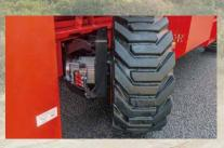
Permanent magnet motor drive, energy efficient, more powerful, excellent waterproofing grade IP67.
