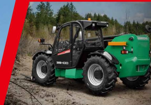
With permanent magnet synchronous motor (PMSM) technology, can reach top speed: 25 km/h, maximum grade ability: 45%, and industry-leading performance in its class.
