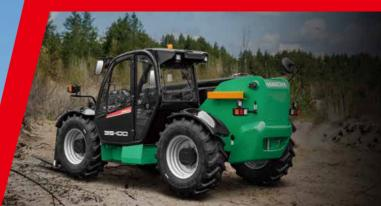
With permanent magnet synchronous motor (PMSM) technology, can reach top speed: 25 km/h, maximum grade ability: 45%, and industry-leading performance in its class.
