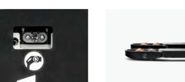
The power plug is fixed on the truck body to avoid damage from battery installment.
