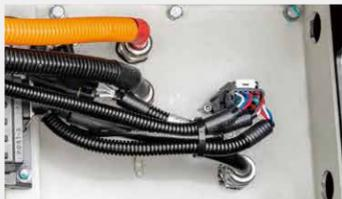
The power plug is fixed on the truck body to avoid damage from battery installment.
