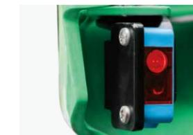
Foot detection sensor - trucks slows down or stops if operator's foot is detected outside of the platform contours [Option].
