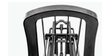
The truck with assembly overhead guard can protect the driver's safety in case of high-position cargo falling.
