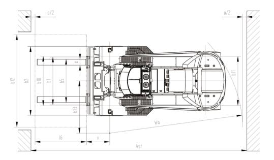
Ast=16+Wa+x+a16: load length a:Clearance(200mm)
