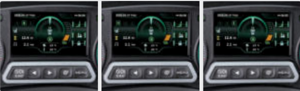
N (Normal) : Same acceleration feel as ICE forklifts H (High) : Implement instant acceleration performance for fast task processing E (Economic) : Smooth acceleration performance with energy efficiency
