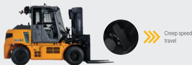
Allows travel at 2.5 km/h without pressing the accelerator
