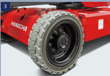
Tires: foam-filled tires with good off-road performance
