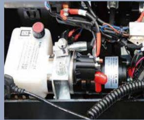
Integrated hydraulic unit, compact structure, less space
